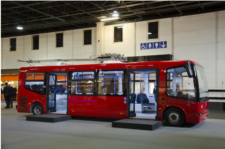
Conversion of an electric midi-bus into trolley-battery charging bus & testing of prototype bus in TROLLEY 2.0 partner cities (Evopro, all cities)
