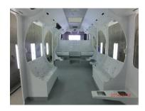
The manufacturing and assembly time can reduce with 223 hours, because the composite sandwich structure give better solution with painting materials. Water resistant and anti vandal.
